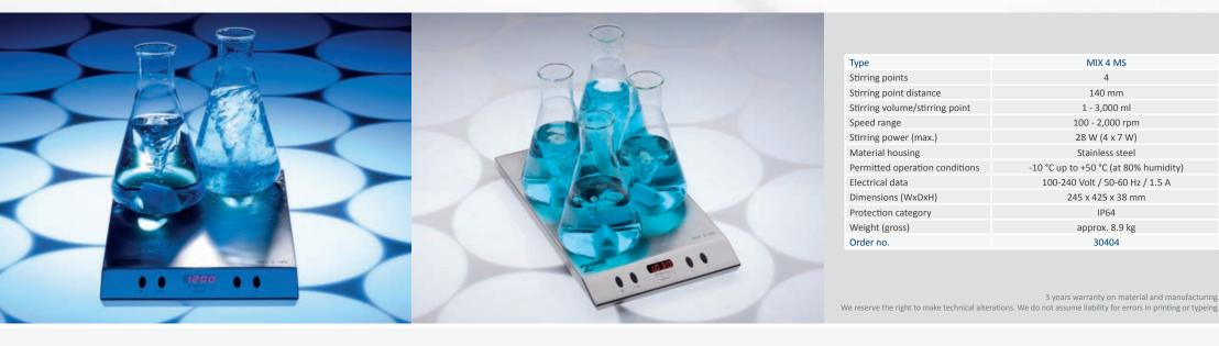
Powerful 4 stirring positions, 100% maintenance-free and wear-free by inductive 2mag-Magnetic-Drive concept, power reserves up to 3,000 ml per stirring point, individual and independent speed setting for each stirring drive (Master-Slave-Technology), also ON/OFF function, synchronous speed mode for all positions, extremely wide speed range of 100 to 2,000 rpm, jerk-free stirring even at low speeds.
